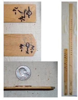
in the hole  $\frac{1}{2}$ " back from the zero mark and your pencil in the 25" hole. If you want a hole that is  $25\frac{3}{4}$ " radius. Put the nail in the -1/4 hole and the pencil in the 26" hole.
