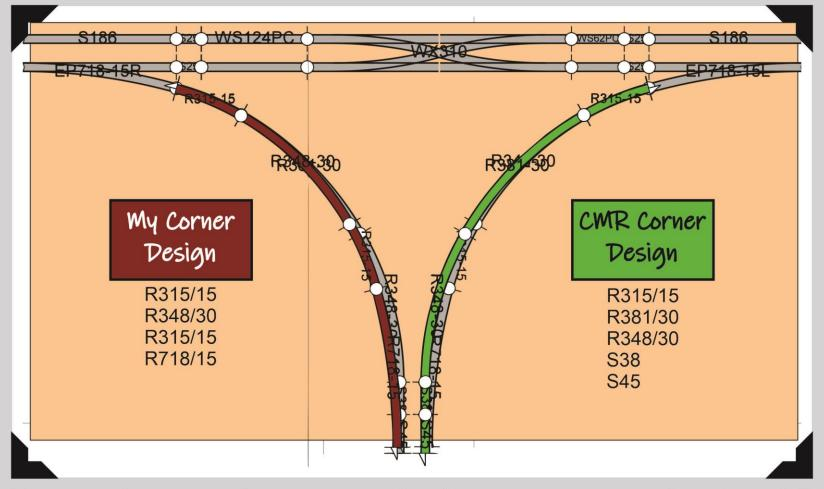
Although the CMR large junction design was the best match yet developed for the large 480 /447mm radius corners I never really liked the corners and the 2 small pieces of straight track required. So I took the curved track from the Super Cross, replaced one #6 turnout with the equivalent 718mm radius 15 degree corner and an accidental improvement resulted.
