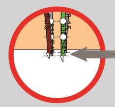
The nose of the junction curves is a few mm too long and the track spacing is narrow in the original design.
