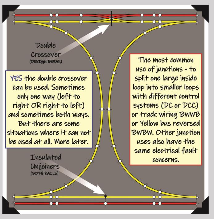
To prevent possible electrical faults between two adjacent inner loops the large ("Branchline") junctions with the straight track between the curves
