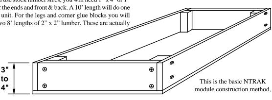
Use sheet rock screws and glue to hold the corner blocks in place. If you fasten the blocks to the end pieces first, the assembly will go easily. I use a "C" clamp to hold the block just so, then put the screws in pre drilled holes and tighten them down. The screws in the front and back pieces should be located so that they don't run into the first set of screws.
