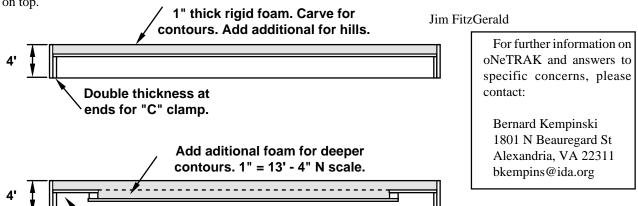
For modules that feature hills and valleys, an alternate construction method will make your project easier. You make the module base 3" high with a full plywood top. Then add 1" of rigid foam to the top of it. The ends are made
